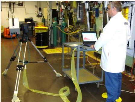
Figure 11. RadSearch measurement in the AGHCF at Argonne National Laboratory. A strong Cs-137 peak and Compton down-scatter are clearly visible in the spectrum displayed on the notebook computer.
