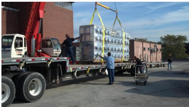
**Figure 3: Loading the First Glovebox for On-site Transport**
