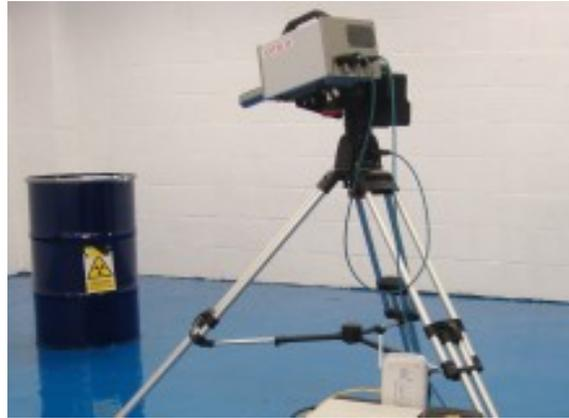
Fig. 3 – RadSearch spectroscopic scintillation gamma camera
