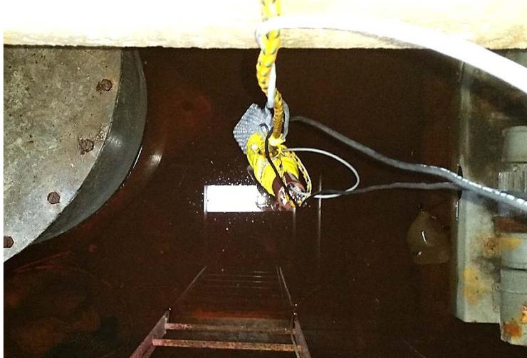
Fig. 1a – Sodium Iodide Detector Suspended in a Sump
