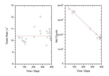
Figure 10. QC charts for the technological combustible QC drum without nuclear sample. Left: Passive Neutron Counting (Passive Background). Right: Active Neutron Counting (Net Counts is equal to Early Gate Counts – Late Gate Counts) (Active Background).
