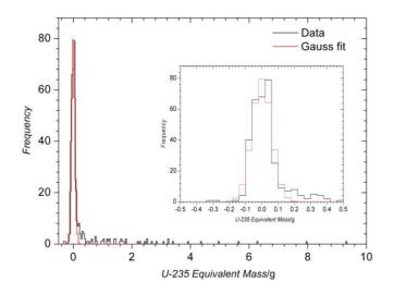
Figure 7. Frequency distribution of U-235 Equivalent Mass (g) for active neutron measurements of technical combustible drums.
