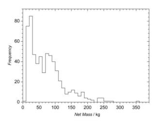
Figure 3. Frequency distribution graph of the Net Mass in kg of the drums measured during WCS pilot operation. No distinction has been made between the different matrices (Technological Combustible, Metal, Cement).
