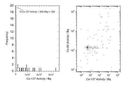
Figure 6. Left: Frequency distribution graph of the Cs-137 Activity (Bq) for the drums measured during WCS pilot operation. One drum with an exceptional high content of 1.1E+8 Bq is not included in the graph. Of the 349 reported SGS measurements 326 of these have an activity below 200 kBq. Right: Graph showing both the Co-60 and Cs-137 activities.
