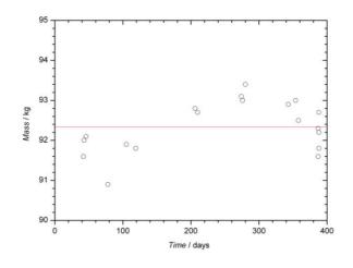
Figure 8. QC chart for the total mass of the QC test drum with technological combustible matrix (including the tare weight of 25.2 kg for the drum and 23.1 kg for the puck on which the 220 litre drums are placed for the movement on the conveyor rollers).
