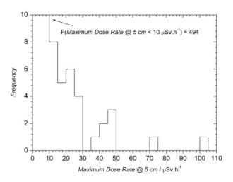
Figure 5. Frequency distribution graph of the Maximum Dose Rate in  $\mu$ Sv.h<sup>-1</sup> of the drums measured during WCS pilot operation. The dose rate is measured at a fixed distance of 5 cm from the surface of the drum.
