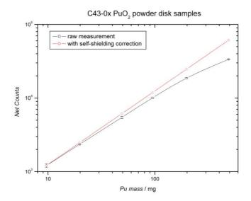
Figure 11. Net counts as a function of total Pu mass for  $PuO_2$  disk standards. A Monte Carlo simulation has been used to model the self-shielding effects for these large standards.
