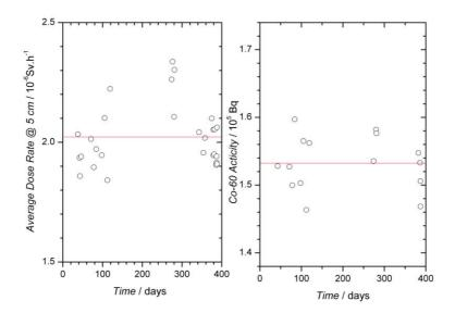
Figure 9. QC charts for the technological combustible QC drum with a small Co-60 source. Left: Average Dose Rate at 5 cm from drum surface. Right: Decay-corrected Co-60 activity from SGS.
