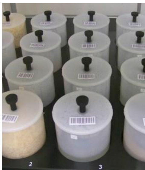
Fig 1. The sample tray with Marinelli beakers containing samples for measurement
