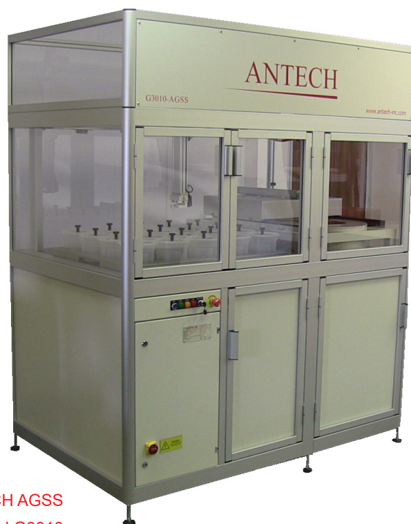
Fig 1. The sample tray with Marinelli beakers containing samples for measurement
