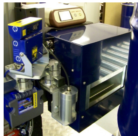
Built-in Geiger-Müller dose rate sensor and waste drum barcode recognition
