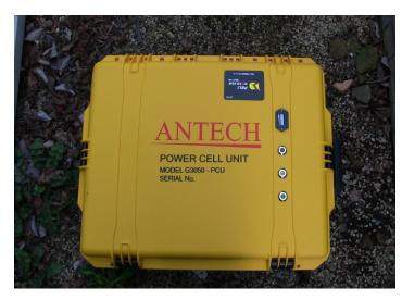
protect the charging electronics. The cases are IP67 rated. On the top surface of the cases, the charge status is provided by LED lights. The cases are provided with collapsible handles and castors, allowing easy transportation over uneven or rough ground.
