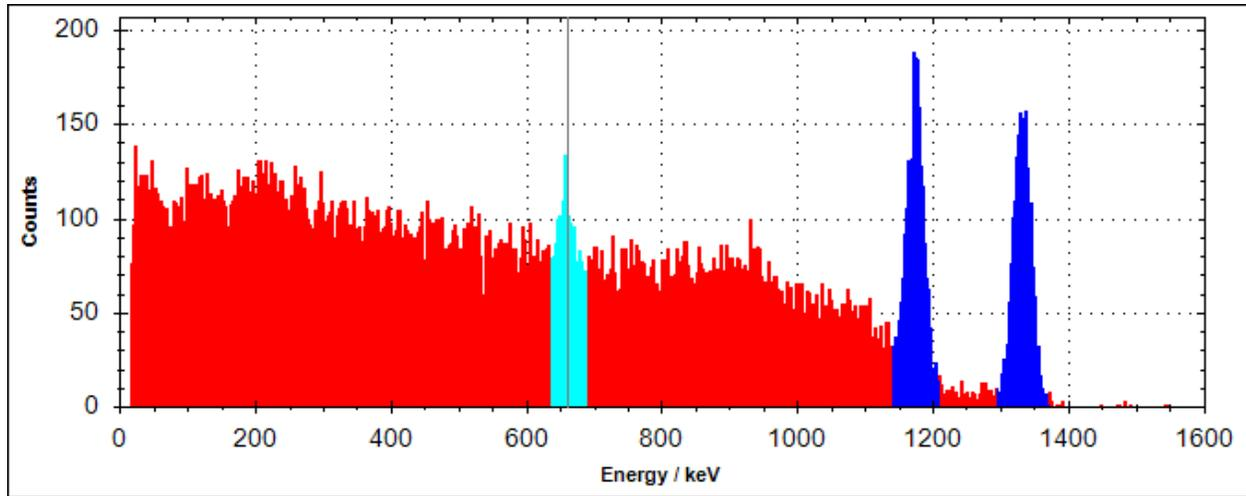
Figure 6. Gamma ray spectrum for the measurement of Waste Container 007, segment 6 (Scan ID= 201401271347), which contains gamma ray peaks for Cs-137 (661.64 keV) and Co-60 (1173.2 keV and 1332.5 keV).
