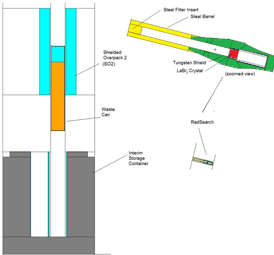
Figure 3. View of a vertical section through the centre of the waste container or can (from the MCNP Model).
