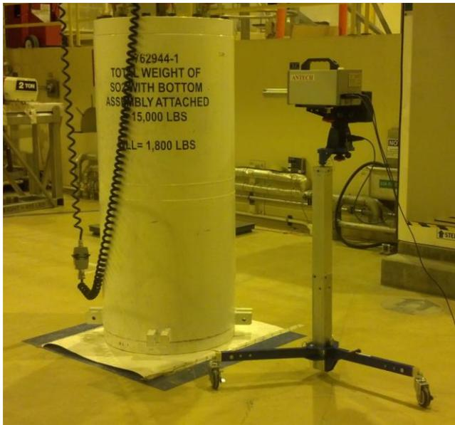
Figure 1. The photograph shows the RadSearch detector head with collimator barrel and pan-tilt mechanism on a mobile stand. The cylindrical object in the photo is a Shielded Overpack 2 (SO2), which is used when a waste container is transferred.
