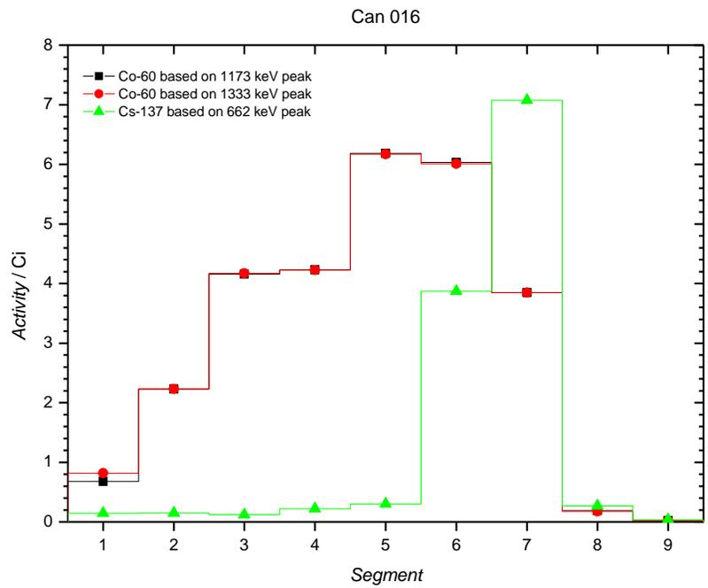
Figure 5. Measured activity (in units of Ci) as a function of the container segments for Waste Container 016.
