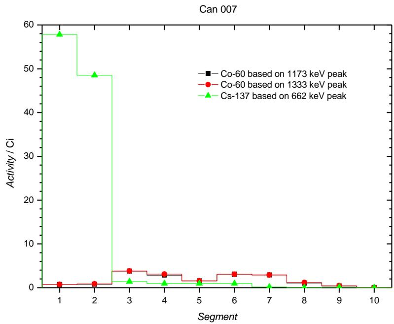
Figure 4. Measured activity (in units of Ci) as a function of the container segments for Waste Container 007.
