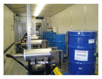
Figure 2. Interior of the ANTECH Gamma Mobile Assay Laboratory (G-MAL) with test drums.
