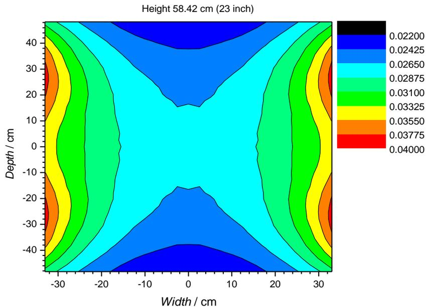
Fig. 7. BLM detection efficiency profile – lower plane at a height of 58.42 cm.
