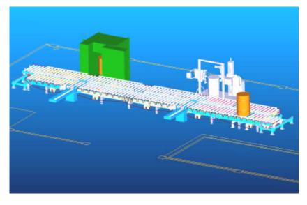
FIG. 2. The Tomographic Segmented Gamma-ray Scanner (TSGS) and DDA assay instruments are coupled to a heavy-duty roller conveyor system, onto which up to 20 waste drums can be loaded.
