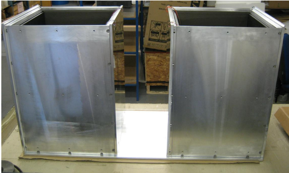
Figure 3. Measurement and reference cells during assembly of the calorimeter
