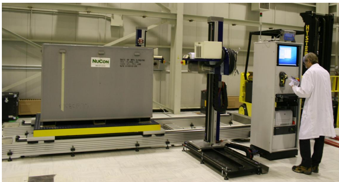
Figure 2. An ANTECH Model 3702 –B25 Gamma Box Counter in operation. The B-25 box is in the load position.
