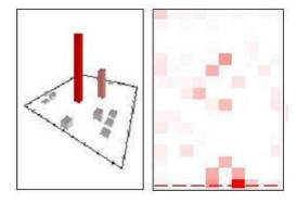
Figure 4. In this figure the results of the tomographic emission-scan of a typical waste drum No. 0059 measured by TGS are displayed. The view on the left shows the magnitude of the activity for Co-60 and its distribution across a plane through the bottom of the drum. The view on the right shows the vertical distribution of activity as seen through one face of the drum. The dashed line is the plane through the bottom of the drum appropriate to the left hand view.
