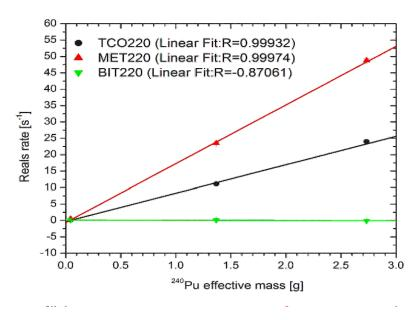
Figure 8. This figure shows calibration curves relating the Reals coincidence rate to the Pu-240 effective mass for three different matrix types.
