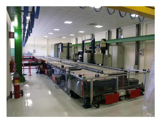
Figure 2. Photograph of the JRC Ispra Waste Characterization System (WCS) showing the tandem conveyor with the gamma measurement station in the foreground and the active/passive differential die-away based neutron measurement station towards the far end of the conveyor.
