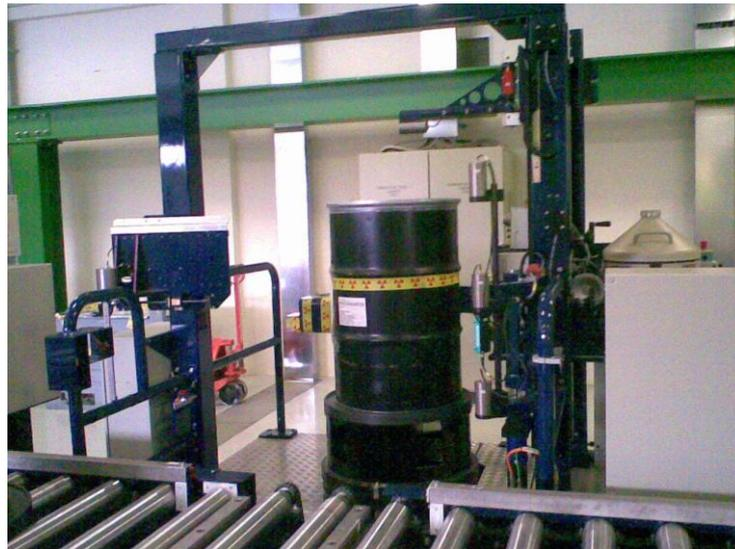
Figure 4. This is a photograph of the Gamma Station showing the dose-rate measurement position in the foreground and the TGS-SGS to the rear.
