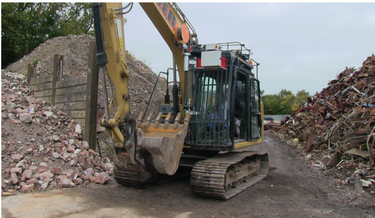
Fig 1. This photograph of the EMBASSY System shows the shielded detector assembly in the upper storage position, rotated towards the front of the operator cab. Note: that the excavator bucket is in the measuring position.
