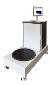
The turntable is designed to accept a 200 L (nominally 600 mm diameter) drum of waste. The turntable mounting plate has locating ring to assist with centralising the drum when it is loaded and to ensure that it stays in position during rotation. The turntable is mounted on a load cell arrangement that has the capability to weigh drums of up to 300 kg. The turntable is fitted with a servo motor and can rotate at a speed of up to 6 rpm to ensure a homogenous scan of the drum.
