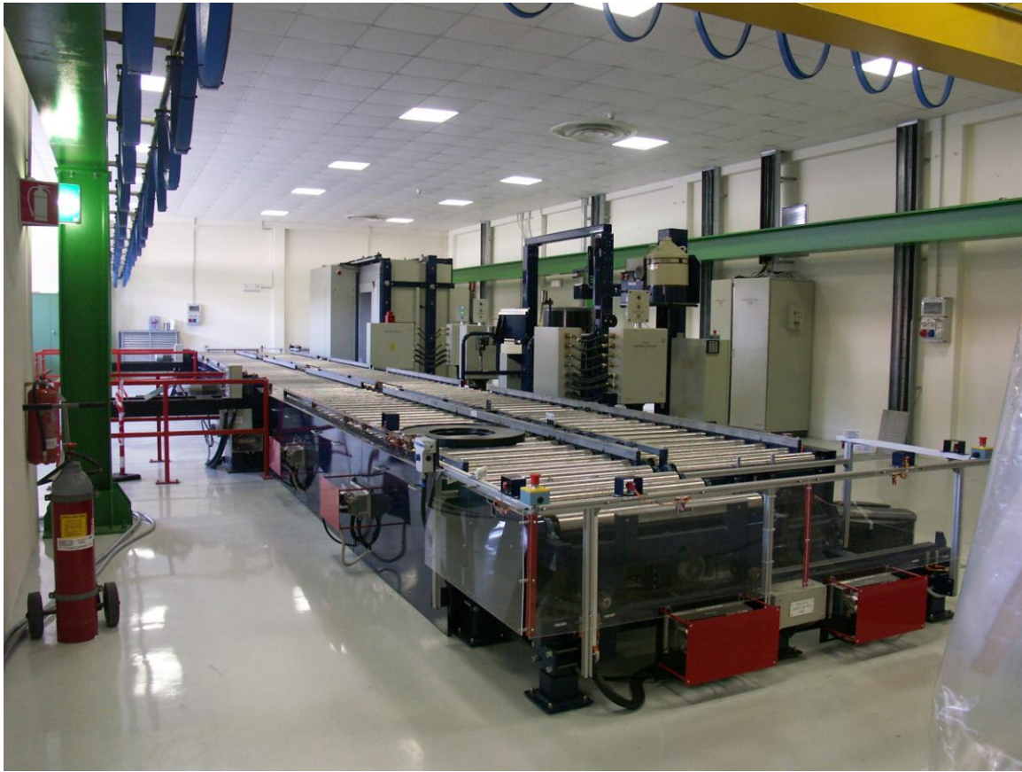
Figure 2. Photograph of the JRC Ispra Waste Characterization System (WCS) showing the tandem conveyor with the gamma measurement station in the foreground and the active/passive differential die-away based neutron measurement station towards the far end of the conveyor.
