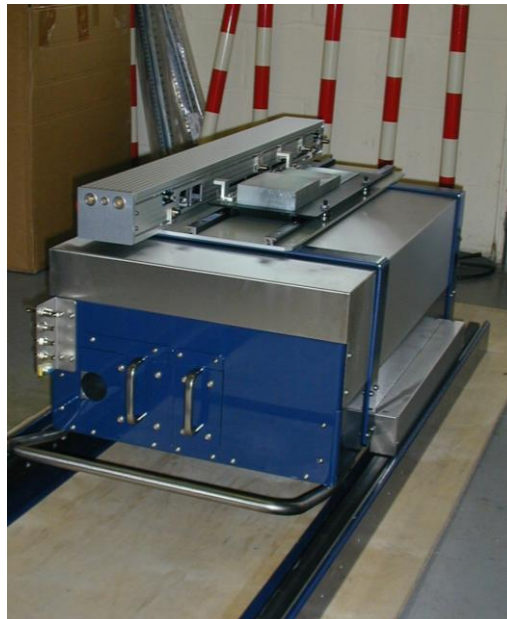
Figure 4. Waste Tray Assay System (WTAS). The stainless steel filters and the filter motion control system can be seen on the top.
