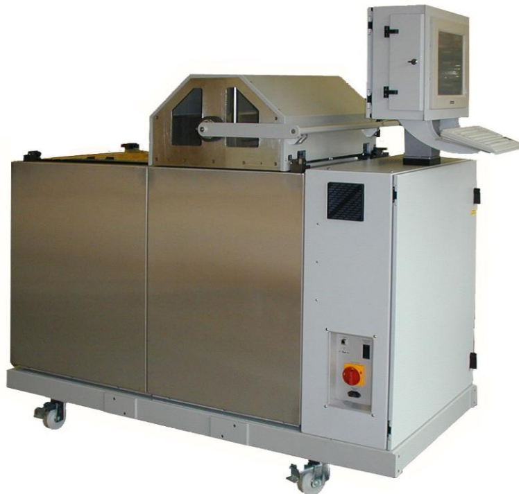
Figure 1. The model 400HF-5300 twin cell heat-flow calorimeter consists of two 53-litre measurement chambers.
