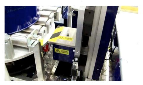
Figure 4. Tungsten shielded transmission source descending into the transmission source safe.
