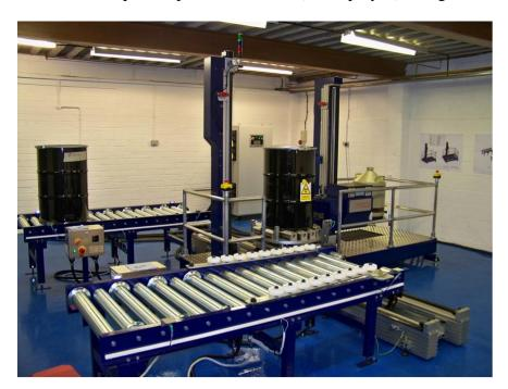
Figure 5. This is a photograph of the model G3250-3850-340 Wide Range SGS-TGS taken part way through a measurement during the FAT. Note that a drum is in the measurement position on the drum rotation platform. The transmission source is deployed and can be seen immediately to the left of the drum just above the mid-height. Another drum (from the previous measurement) is located on the output roller conveyor. The drum centering guides can be seen on the input roller conveyor in the foreground.
