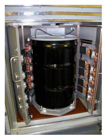
Fig. 3. Drum calorimeter with drum inserted into the octagonal heat sink chamber assembly in the open or loading/unloading position.
