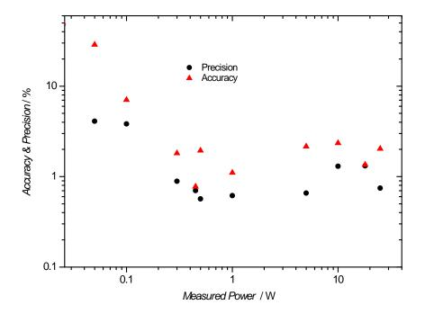
Fig. 9. The precision and accuracy (deviation) of the measured drum thermal power as a function of applied electrical power is plotted as percentage values on a log – log scale.
