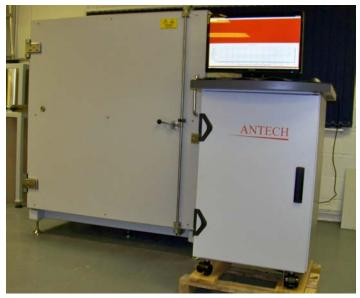
Fig. 1. Model CHF550-20800 Heat-flow Drum Calorimeter.
