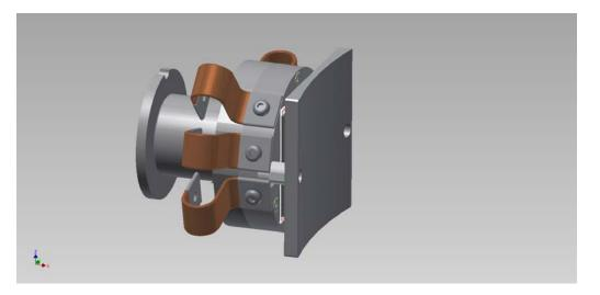
Fig. 2. Thermopile Heat-flow Sensor Assembly (TSA).
