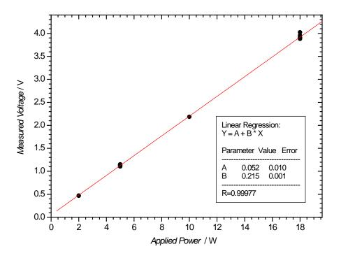
Fig. 5. Drum Calorimeter high power calibration data for thermal powers up to 18.0 Watt.
