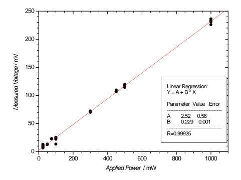
Fig. 4. Drum Calorimeter low power calibration data for thermal powers up to 1.0 Watt showing the measured output voltage from the TSA units plotted as a function of the electrical power applied to the heating element in the test and calibration drum. Note that the calibration is linear due to the linear response of the heat-flow sensors.
