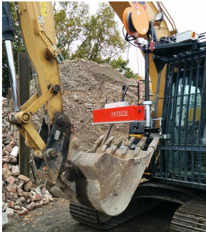
Fig. 5. EMBASSY mounted on an excavator. The detector is in the measurement position.
