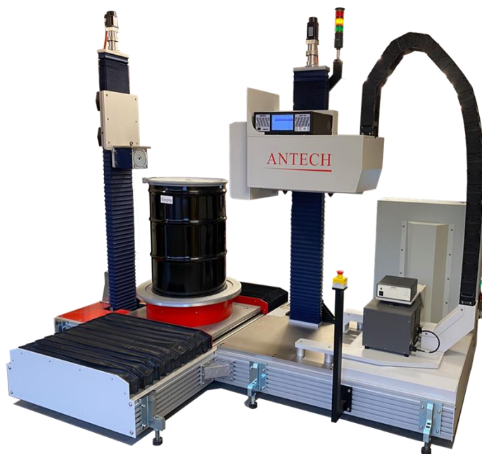
Fig. 1. UDASS with 200 litre waste drum in the measurement position.
