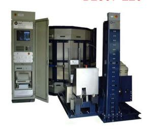
User-friendly Windows software controls the semi-automatic loading of 220 litre (55 gallon) drums and the gamma ray and neutron data acquisition and analysis algorithms. The neutron instrument determines the Pu-240 effective mass (<sup>240</sup>Pu<sub>effective</sub>) and the high purity germanium (HPGe) gamma ray scanning instrument determines the Pu (and U) isotopic ratio data. This data is combined to determine the mass of all of the individual plutonium (and uranium) isotopes.
