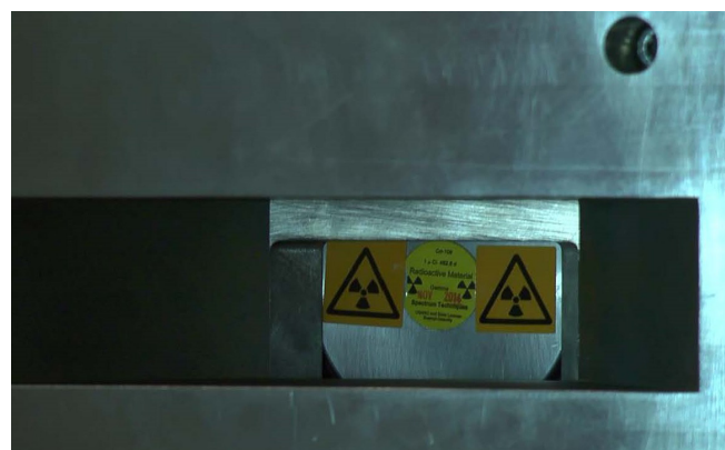
Fig 4: The collimator opening and filter revealing the detector head
