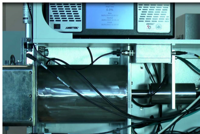
Fig 2: External casing removed to show the shielded detector
