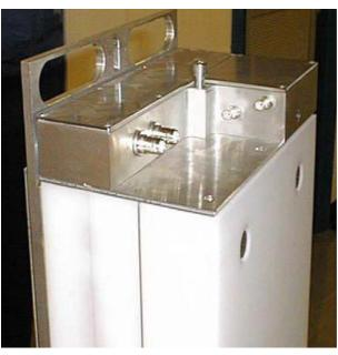
Counter by coaxial signal and Low and High Voltage power cables. The N2000 contains circuitry that provides and monitors the high voltage power supply for the <sup>3</sup>He tubes and the low voltage power supply to provide power to the head amplifier.
