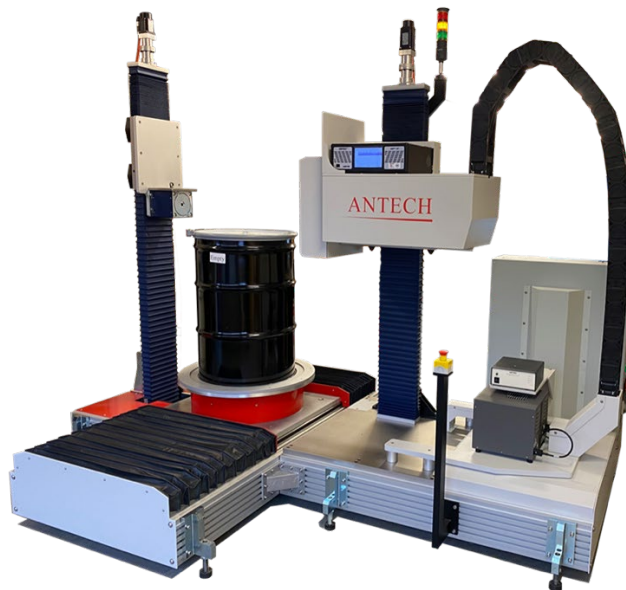
Fig. 1. UDASS with 200 litre waste drum in the measurement position. The transmission source housing can be seen attached to the pillar on the left and the HPGe high efficiency gamma ray detector is located in the housing attached to the pillar on the right of the photo.
