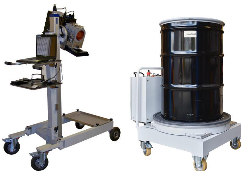
Fig. 3. IMAGE may include the CHARMS detector (the IDM-200-V) deployed on the ANTCart mobile trolley.
