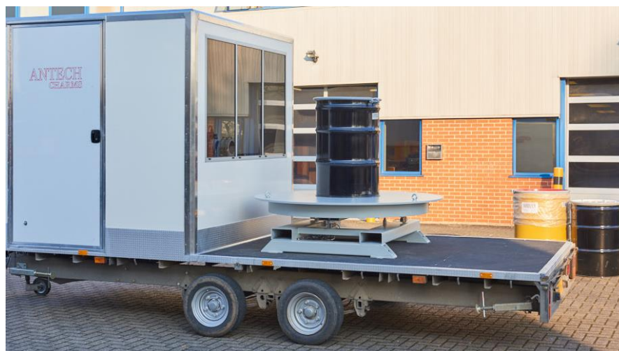
Fig. 2. CHARMS measuring a 55-gallon (200 litre) drum.
