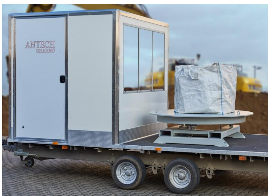
Fig. 1. CHARMS measuring a one cubic metre 'builders' bag' in the field.
