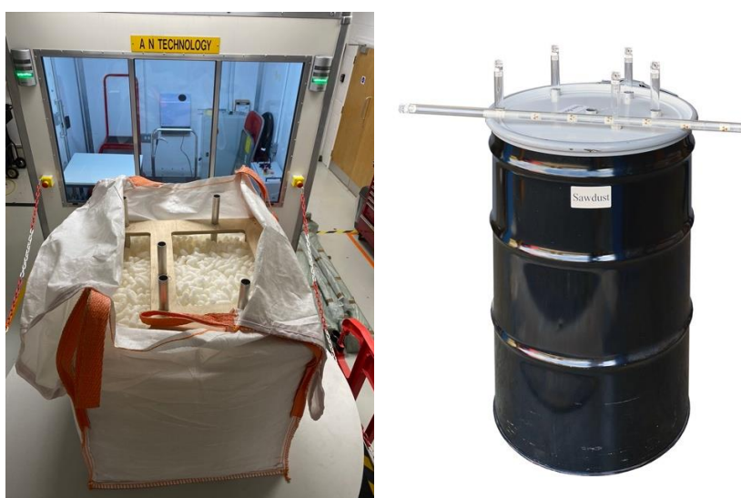
Fig. 5. This photograph shows a test drum with re-entrant tubes into which rod sources can be placed. Also shown is a view of a test bag on the CHARMS turntable. Note the location of re-entrant tubes inserted into the bag, into which rod sources may also be placed for testing.
