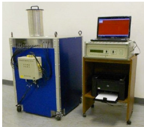
The Model B2308 Plutonium Scrap Multiplicity Counter with an ANTECH Model N1003 Time Correlation Analyser
