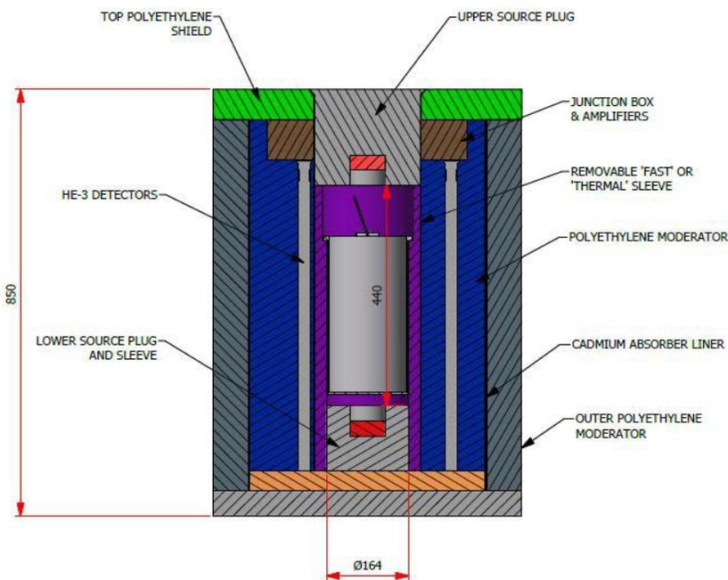
Fig. 2. Cross-section view of the Neutron Measurement Subsystem.
