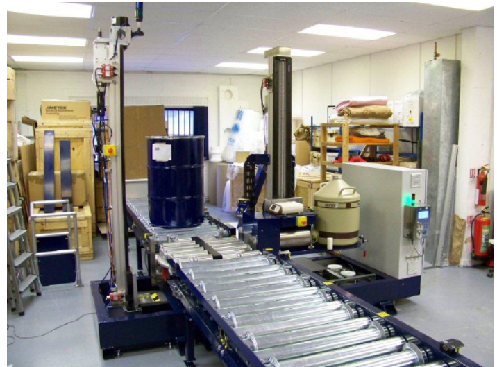
Input-output conveyor used for Wide Range SGS
