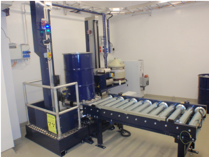
Reversing input-output conveyor on SGS system
