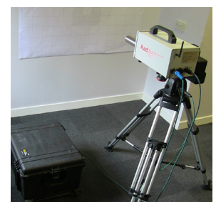
Fig 2. The ANTECH G3050 RadSearch Remote showing the antenna for wireless communication and the "hot-swap" battery pack
