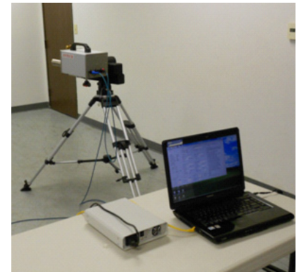
Fig 3. RadSearch deployed showing PSU and ruggedized notebook computer
