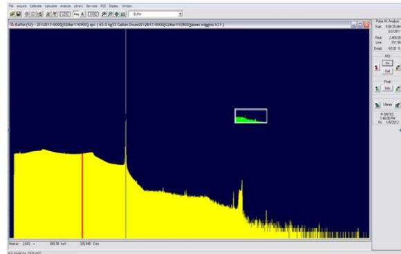
Figures 6a and 6b. Cs-137 indicator @ 661 keV and sum peak @ 1323 keV, no Pu indicated; however, the passive neutron measurement reports 22.27 mg Pu-240 related to 0.167 g total Pu in the sample.
