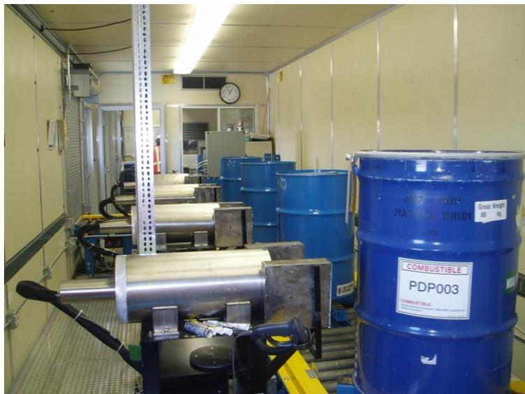
Figure 2. Interior of the ANTECH Gamma Mobile Assay Laboratory (G-MAL) with test drums.
