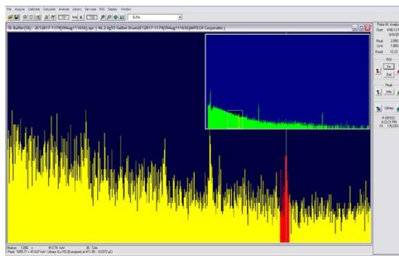
Figures 11a and 11b. Pu, Am, and U present; LLW characterization
