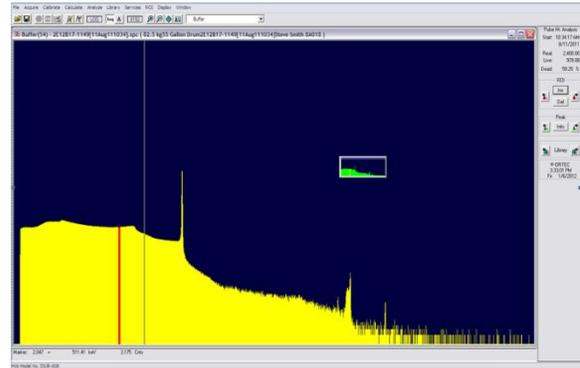
Figures 5a and 5b. Cs-137 indicator @ 661 keV and sum peak @ 1323 keV, no Pu indicated and the neutron measurement reports Pu-240 below detection limit. Lower detection limit relates to 0.045 g total Pu in the sample.
