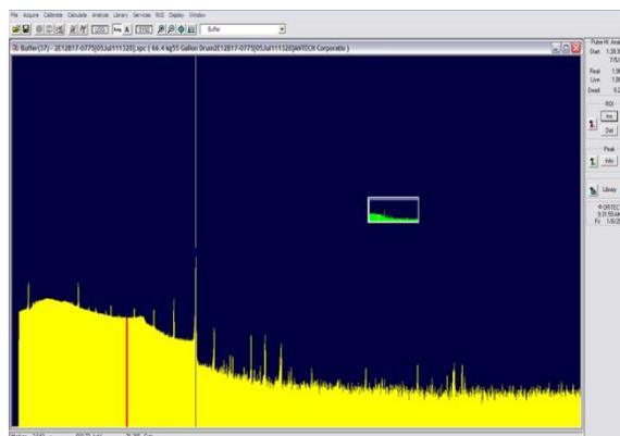
Figures 9a and 9b. High Cs-137, U-233 indicator @ 440 keV, Th-232 indicators @ 969 and 911 keV
