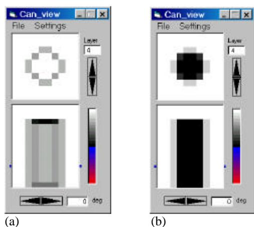
FIG. 3. Base images of the (a) can and (b) UO<sub>2</sub> generated by the ADD-A-CAN software, as viewed using the ANVIEW image viewing software. These are used as constraints in transmission imaging. The can image on the left corresponds to the **SHOW U** command listing in Fig. 2.
