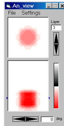
FIG. 5. A constrained emission image of 186-keV gamma rays from standard U49.
