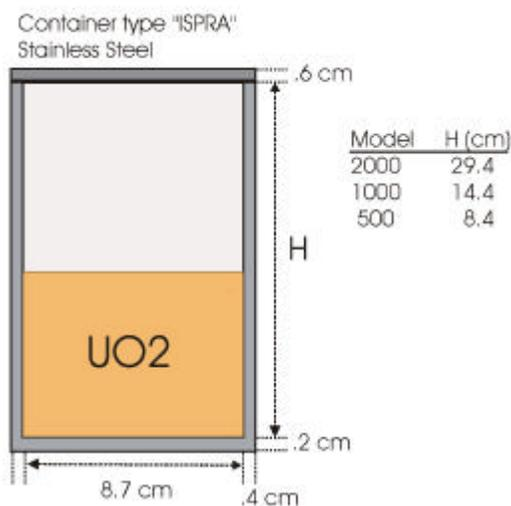
FIG. 1. “ISPRA” cans for storage of UO<sub>2</sub>. The cans come in three sizes of varying height and volume, but with the same diameters. The approximate maximum volumes of UO<sub>2</sub> that the cans will hold are 1.7-L (model 2000), 0.84-L (model 1000), and 0.49-L (model 500). The UO<sub>2</sub> fill height is variable.
