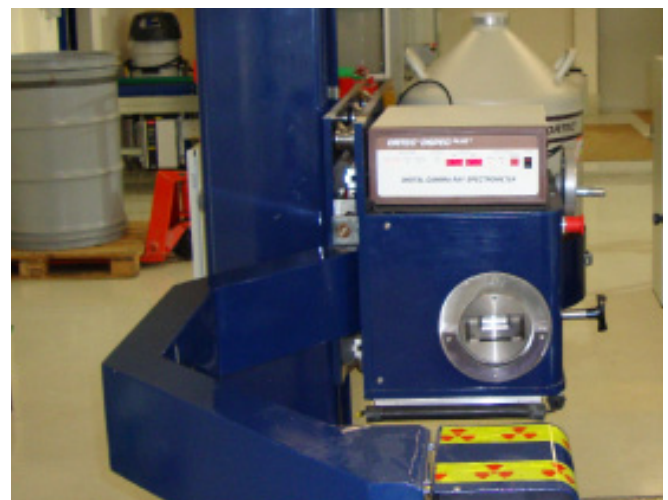
Side profile showing the transmission source arm and detector
