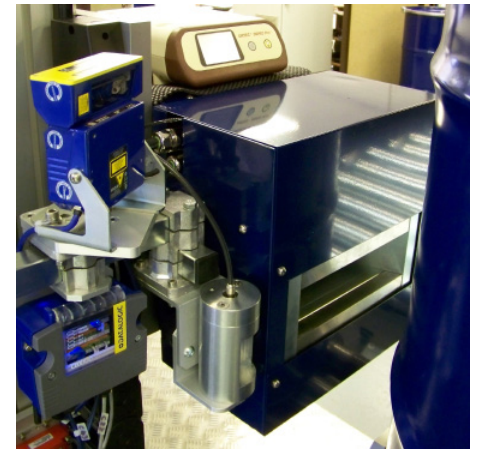
Built-in Geiger-Müller dose rate sensor and waste drum barcode recognition
