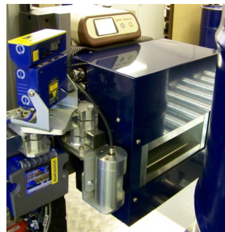
Built-in Geiger-Müller dose rate sensor and waste drum barcode recognition
