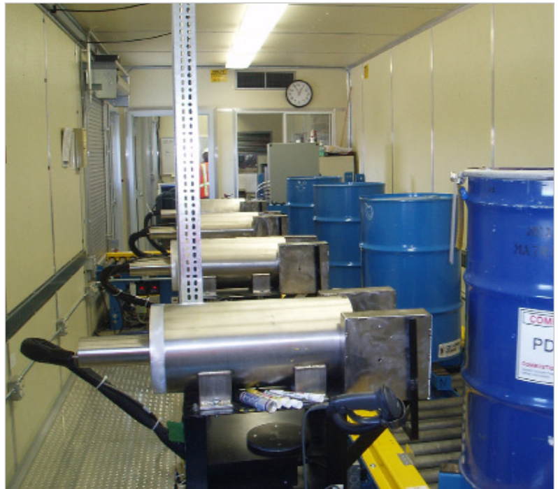
Image of the Far Field Gamma systems used in the ANTECH Gamma Mobile Assay Laboratory (G-MAL). In this example the detectors are electro-mechanically cooled and each detector also has a lead shadow shield.
