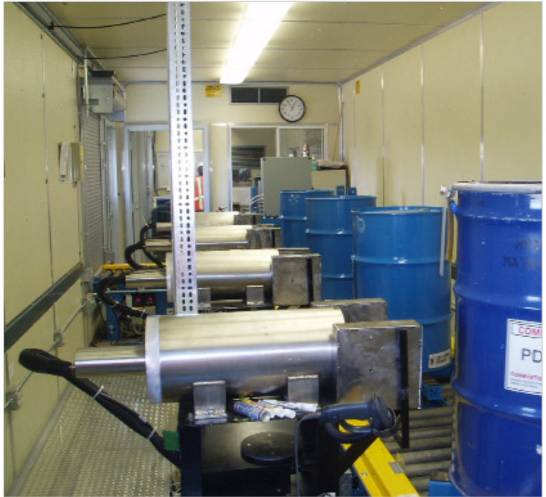
Image of the Far Field Gamma systems used in the ANTECH Gamma Mobile Assay Laboratory (G-MAL). In this example the detectors are electro-mechanically cooled and each detector also has a lead shadow shield.
