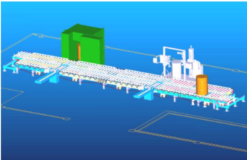
FIG. 2. The Tomographic Segmented Gamma-ray Scanner (TSGS) and DDA assay instruments are coupled to a heavy-duty roller conveyor system, onto which up to 20 waste drums can be loaded.
