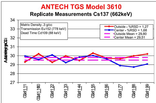
**Figure 6-Replicate Measurements of a 30µCi source (TGS)**
