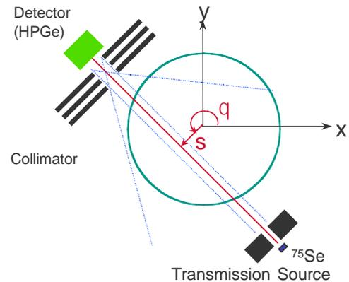
Figure 2 - TGS measurement geometry.
