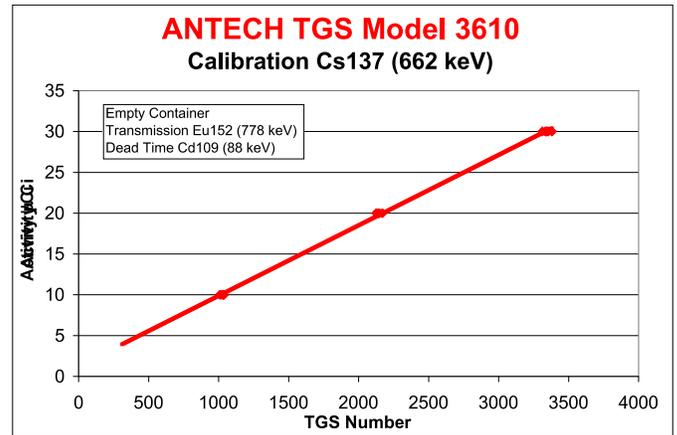
Figure 4 - Calibration of Tomographic Gamma Scanner
