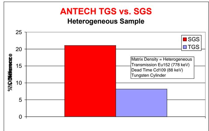
**Figure 8 – TGS & SGS Errors in Heterogeneous Matrix**
