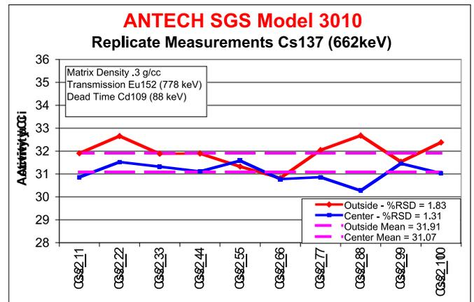
Figure 5–Replicate Measurements of a 30μCi source (SGS)
