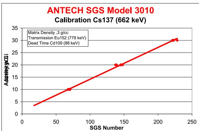
Figure 3 – Calibration of Segmented Gamma Scanner
