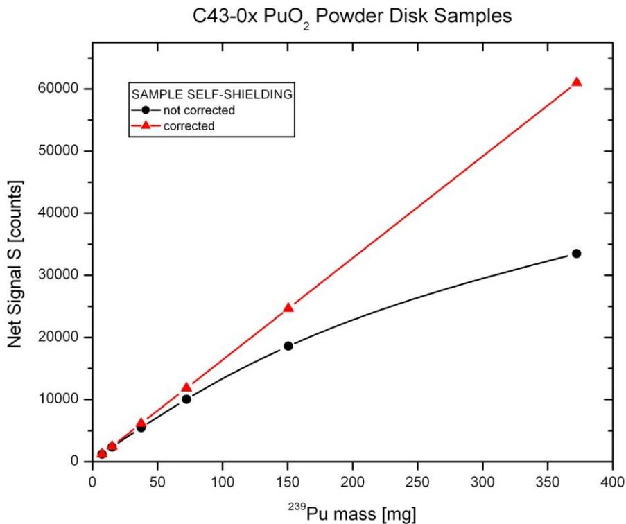
**Figure 10.** Active neutron differential die-away results for the measurement of a variety of PuO<sub>2</sub> powder disk samples. The results of an MCNP simulation to correct for self-shielding are also plotted. The relevant data is tabulated in Table 1.
