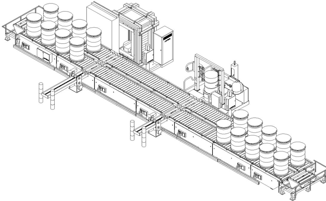
**Figure 1 – Combined Technology Automated Waste Characterisation System**
