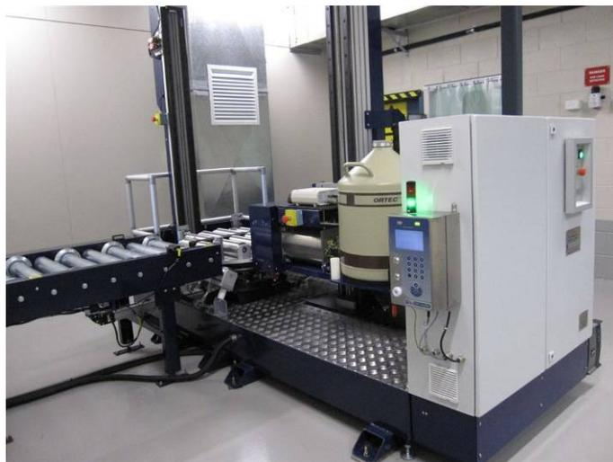
Figure 1 Photograph of the ANTECH WR-SGS installed at ANSTO.
