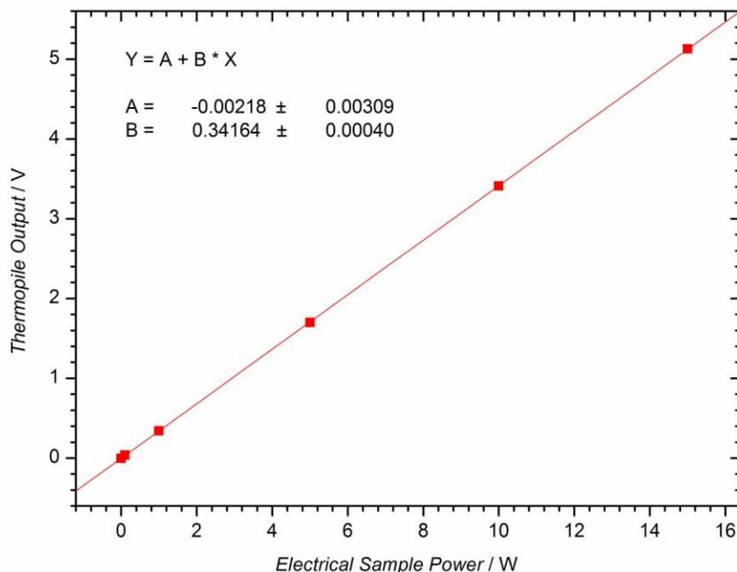
Fig. 7. Thermopile heat-flow sensor output voltage is plotted as a function of applied electrical sample power.
