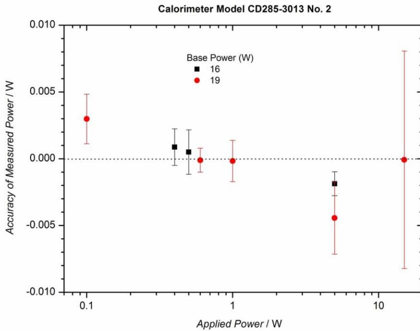
Fig. 5. The accuracy (deviation) of the measurement sample thermal power as a function of applied electrical power is plotted as absolute values.
