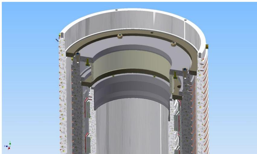
Fig. 2. A cross section view of the top of the calorimeter thermal element.
