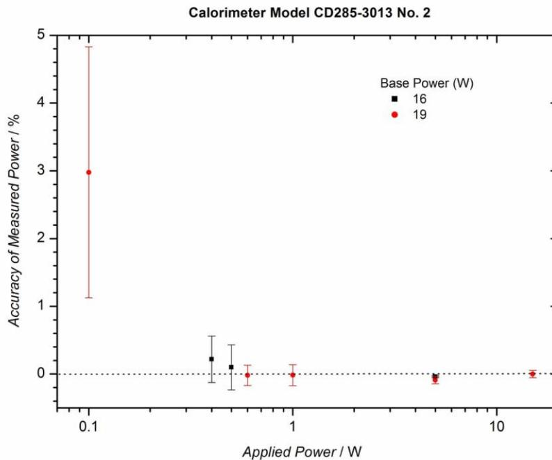
Fig. 6. The accuracy (deviation) of the measurement sample thermal power as a function of applied electrical power is plotted as percentage values.
