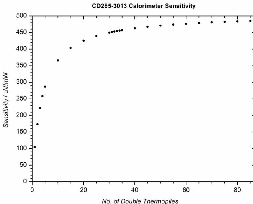
Fig. 3. Using a heat-transfer model, the calculated calorimeter sensitivity is plotted as a function of the number of double (two fixed together) differential thermopile heat-flow sensor assemblies that are positioned in the gap between the inner and middle cylinders.
