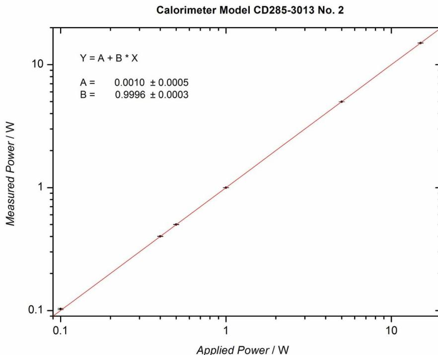
Fig. 4. Isothermal Calorimeter calibration data showing the measured calorimeter sample thermal power plotted as a linear function of applied sample electrical power provided by an electrical heat standard sample container, for calorimeter No. 2.
