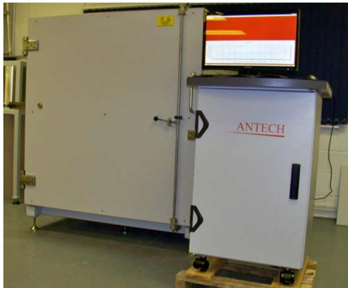
Fig. 1. Model CHF550-20800 Heat-flow Drum Calorimeter.
