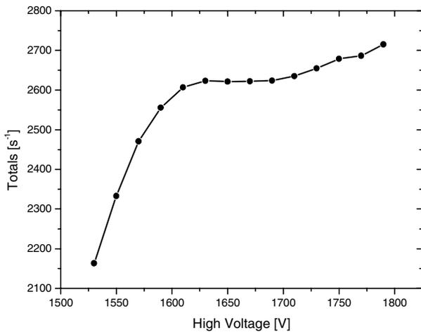
Fig. 2. Typical High Voltage Bias Curve for Model 2200.
