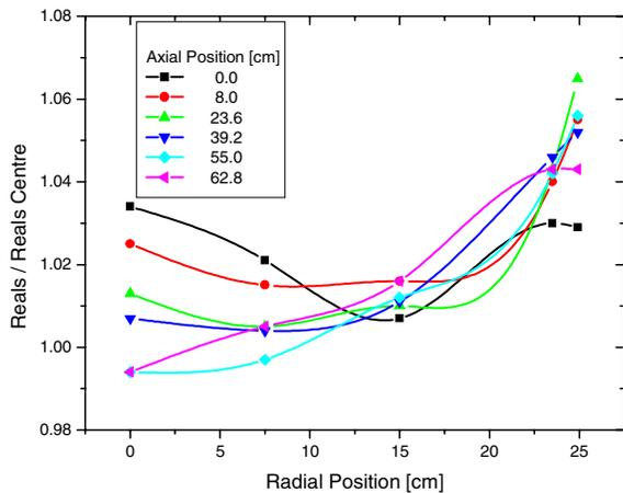
Fig. 5. Radial variation in the coincidence response in a moderating waste matrix of Model 2200, at a number of axial positions.
