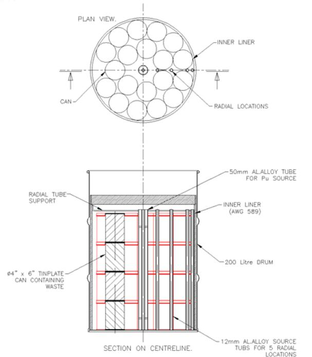
Fig. 4. Apparatus used to measure axial and radial response
