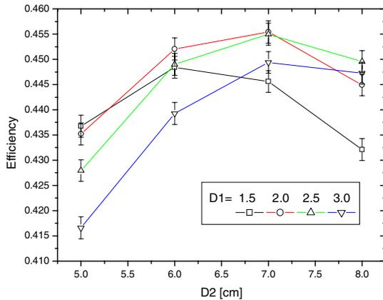
Fig. 8. Simulation results for the detection efficiency of a  $^{252}\text{Cf}$  point source placed in the centre of the measurement cavity as a function of D2 for a number of values of D1.
