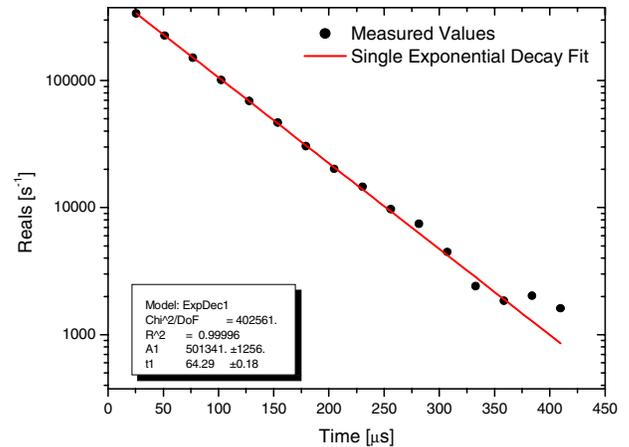
Fig. 3. Typical Die-away Curve for Model 2200
