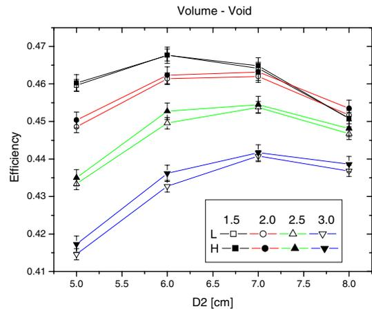
Fig. 9. Simulation results for the detection efficiency for Low (L) and High (H) Burn up Pu waste as a function of D2, for a number of D1 values. The configuration was for a volume source inside an empty drum.
