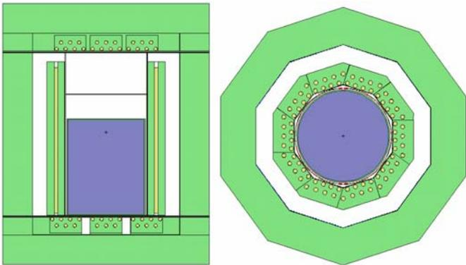
Fig. 6. Model 2203 Neutron Drum Monitor (MCNP Plot), configured for 200 litre waste drum.
