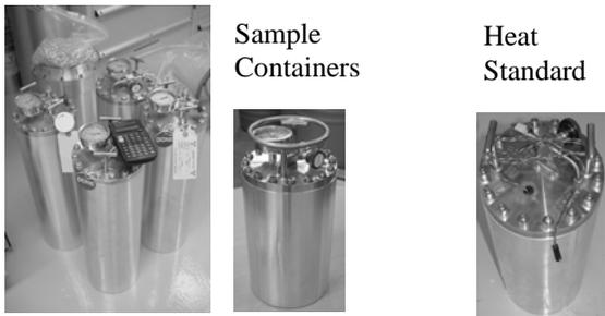
Fig. 2. Photographs of tritium sample containers and the electrical heat standard.
