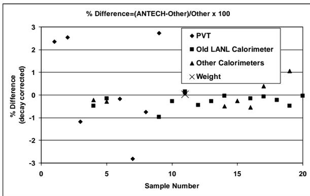
Fig. 7. Cross-comparison of data for unknown samples.
