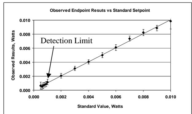
Fig. 4. Endpoint results at the instrument detection limit.
