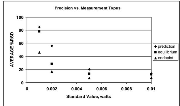
Fig. 3b. Precision results at lower Wattages.
