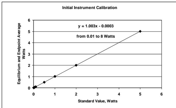
Fig. 5. Initial calibration results for the ANTECH calorimeter.
